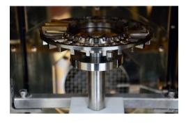
desired temperature (each sample can have individual temperature), and after the soaking time past, tested within the described 5 seconds since removal from the chamber. The test data are transmitted automatically to customers HOST system.
