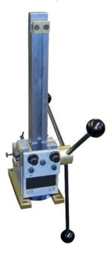
The Model 35 Hand Operated Charpy Notch Broaching Machine is designed for test houses and laboratories, which are producing small batches of test pieces in carbon steels, easily machined low alloy steels, non-ferrous and plastic materials.
