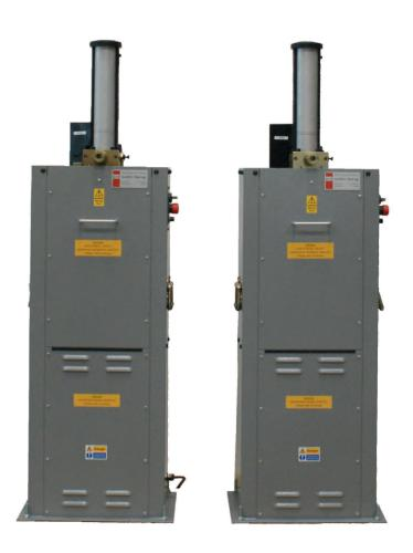
**Motorized Charpy Broaching Machine** is a self-contained floor mounted unit, specially designed for cutting Charpy and Izod 'V' and 'U' notches in premachined standard 10mm square, sub-size and 0.45" diameter specimens.
