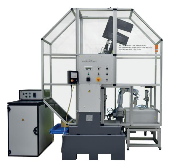
**The Environmental Chamber** is designed for Temperatures from -180°C via LN2 up to +300°C. The specimen magazine can be entered from the front door. The specimens are picked by robot from the top through the round chamber opening (griper entry port).
