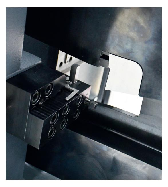
The IZOD specimen support includes the quick specimen centring device for easy specimen loading and clamping.
