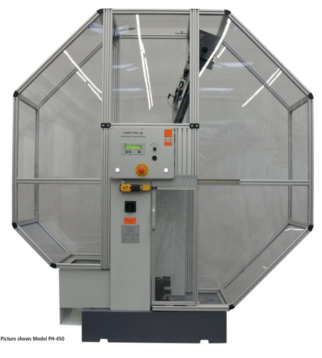
The impact tester is composed of a sturdy, vibration-damping steel cast iron metallic frame with high stiffness on a lower massive structure able to ensure a steady base.
