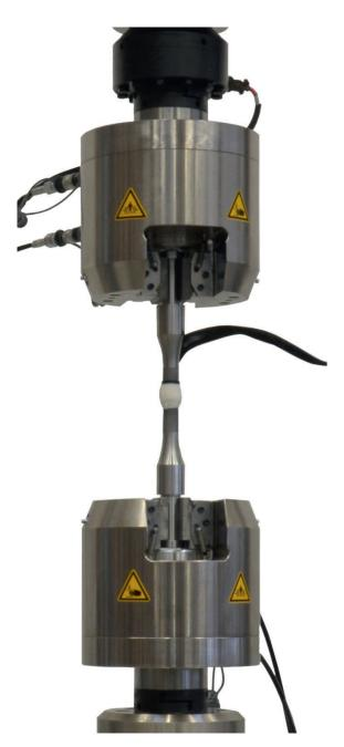
The grip is designed such that there is no backlash while passing through zero load which makes them the best solution for many tests including those with tension-compression loading.
