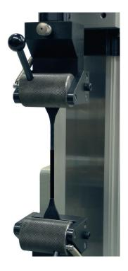
The self-tightening roller grips are easy & quick to operate grips for tensile testing of rubber, flexible polymers and plastics, elastomers, thin sheets, films, bio-textiles and other flexible materials exhibiting a large reduction in cross-section area during testing.
