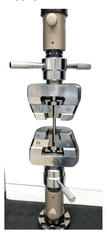
These self-tightening 300 kN grips provide proportional gripping force increase that minimice specimen slippage without the need for pneumatic or hydraulic actuation. A low initial gripping force is applied perpendicular to the flat or round specimen via the handle. The open front design makes specimen loading and changing of the inserts quick and easy.
