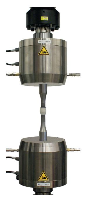
This hydraulically actuated grips hold a specimen during testing with a constant gripping force regardless of the applied axial test force. The short and stiff grip design minimize lateral movement and provides superb alignment and repeatability that minimize the introduced bending strain that can invalidate your test results.
