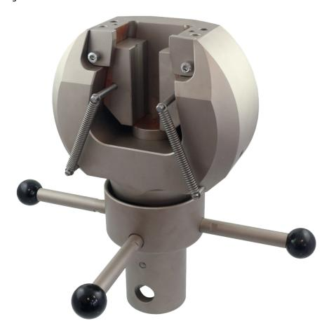
These self-tightening grips are available up to 250 kN and provide proportional gripping force increase that minimice specimen slippage without the need for pneumatic or hydraulic actuation. A low initial gripping force is applied perpendicular to the flat or round specimen via the handle. The open front design makes specimen loading and changing of the inserts guick and easy.
